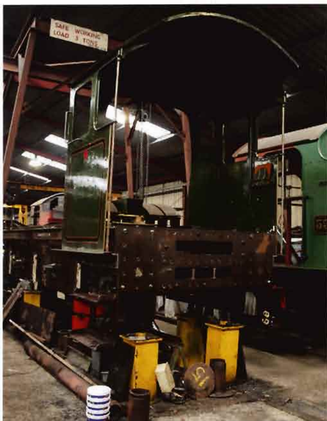
Landmark: the cab and main frames are united.
