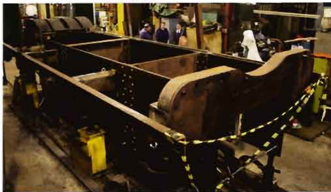
6880's smokebox saddle bracket is now in place.
