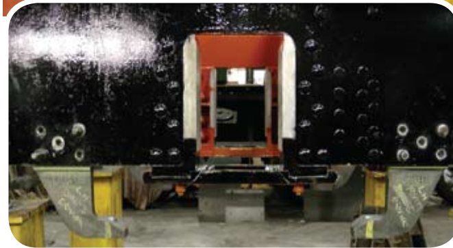
This view shows the centre horn guides with two of the dog legs fitted. These will carry the spring hangers. Dave Owen.
