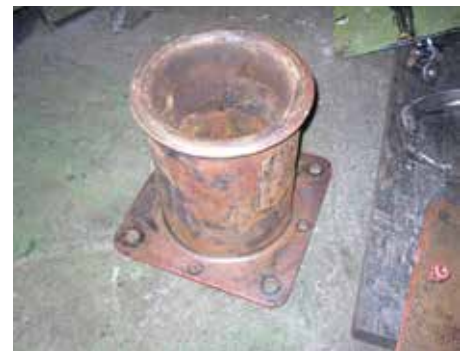
One of the buffers, cleaned and ready for painting
