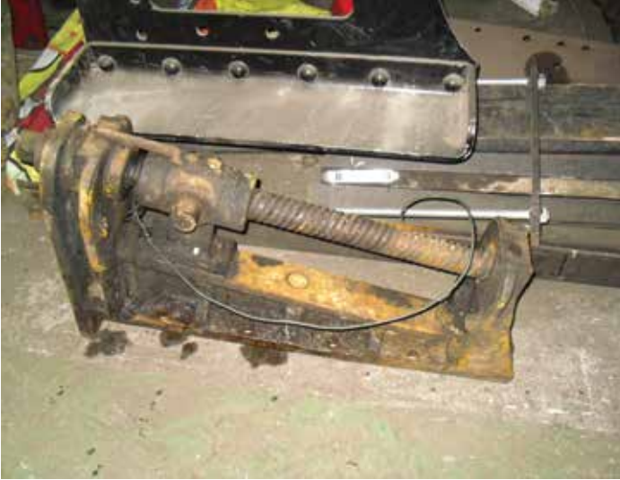
No. 6880's crew reverser prior to refurbishment
