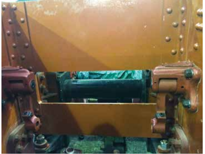
A view inside the frames showing components for the inside motion
