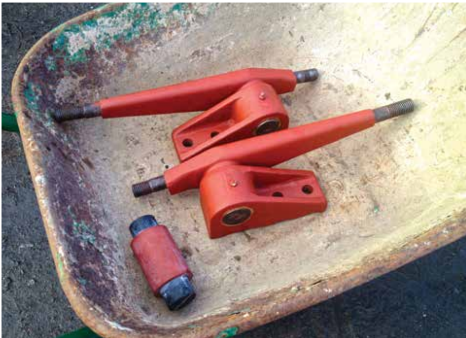
New brake cylinder brackets for 6880
