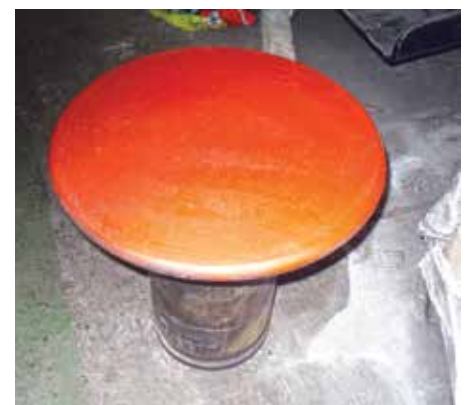
One of the new buffer faces prior to reassembly and fitting to No. 6880
